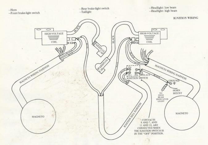
IGNITION. CAPACITOR CHARGING CURRENT: FROM MAGNETO THROUGH BLUE WIRE IN MAGNETO WIRING HARNESS TO UPPER LUG ON HIGH-VOLTAGE COIL. DISCHARGE TIMING PULSE: FROM MAGNETO THROUGH BLACK WIRE IN MAGNETO WIRING HARNESS TO LOWER LUG ON HIGH-VOLTAGE COIL. IGNITION KILL: CHARGING CURRENT GOES FROM MAGNETO THROUGH MAGNETO WIRING HARNESS TO HIGH-VOLTAGE COIL (BLUE WIRE); THROUGH IGNITION KILL HARNESS TO IGNITION SWITCH (BLUE WIRE); TO GROUND AT HORN MOUNT (BLACK WIRE), SHORT-CIRCUITING THE CHARGING CURRENT.
