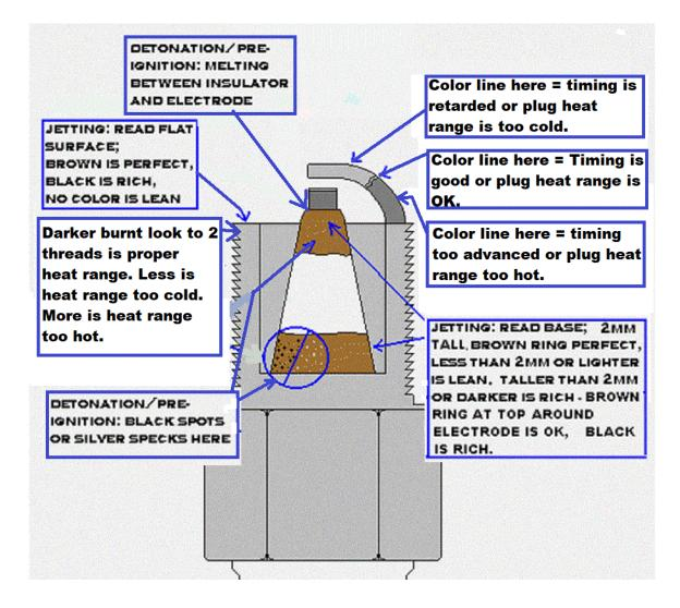
This is what your plug should look like down inside. I cut the metal off so you could see an example that looks like the plug drawing. You will need a strong light to see down inside the plug at the lower fuel mixture ring. It's very hard to take a picture of this but you can get the idea. If the color is lighter or not as tall it's too lean. If the color is darker or taller it's probable too rich but on the safe side. You can also see the color at the top by the center electrode.
